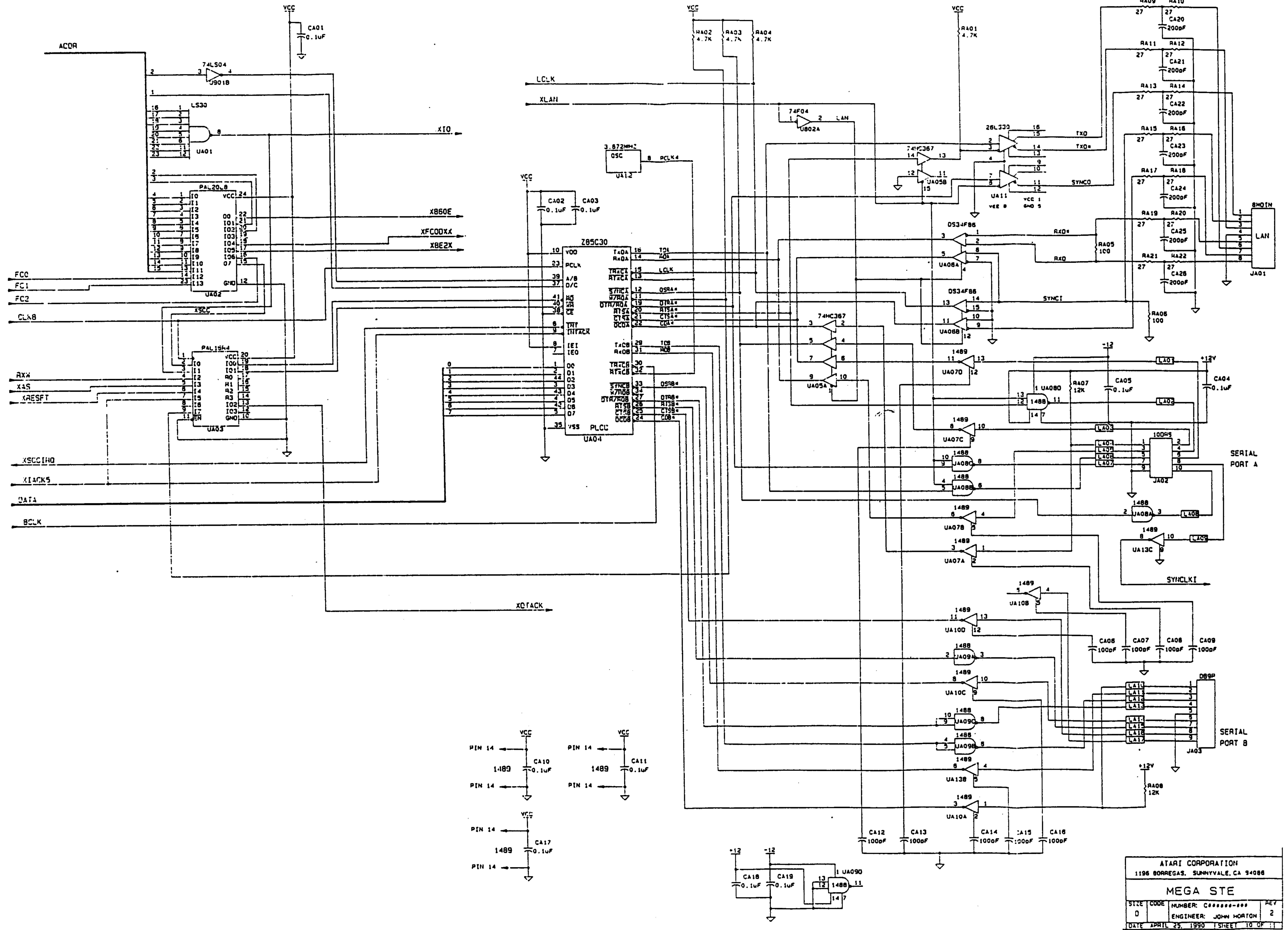
UB01 NEED NOT BE INSTALLED IF UB02 IS NOT PRESENT
