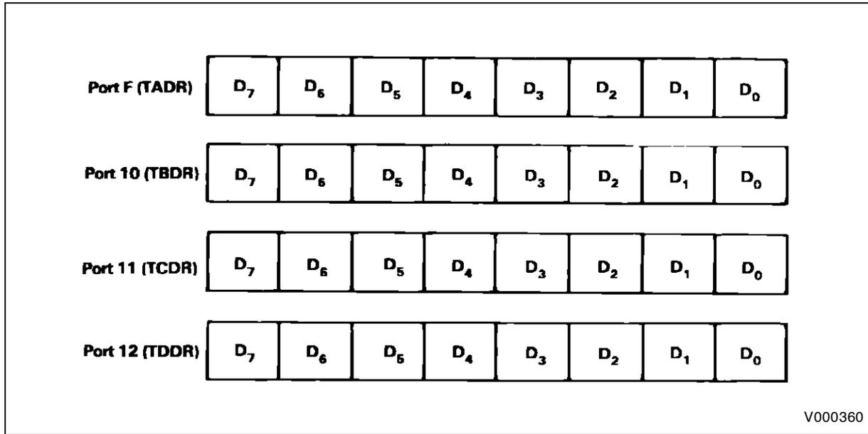
Figure 14 : Timer C and D Register.
