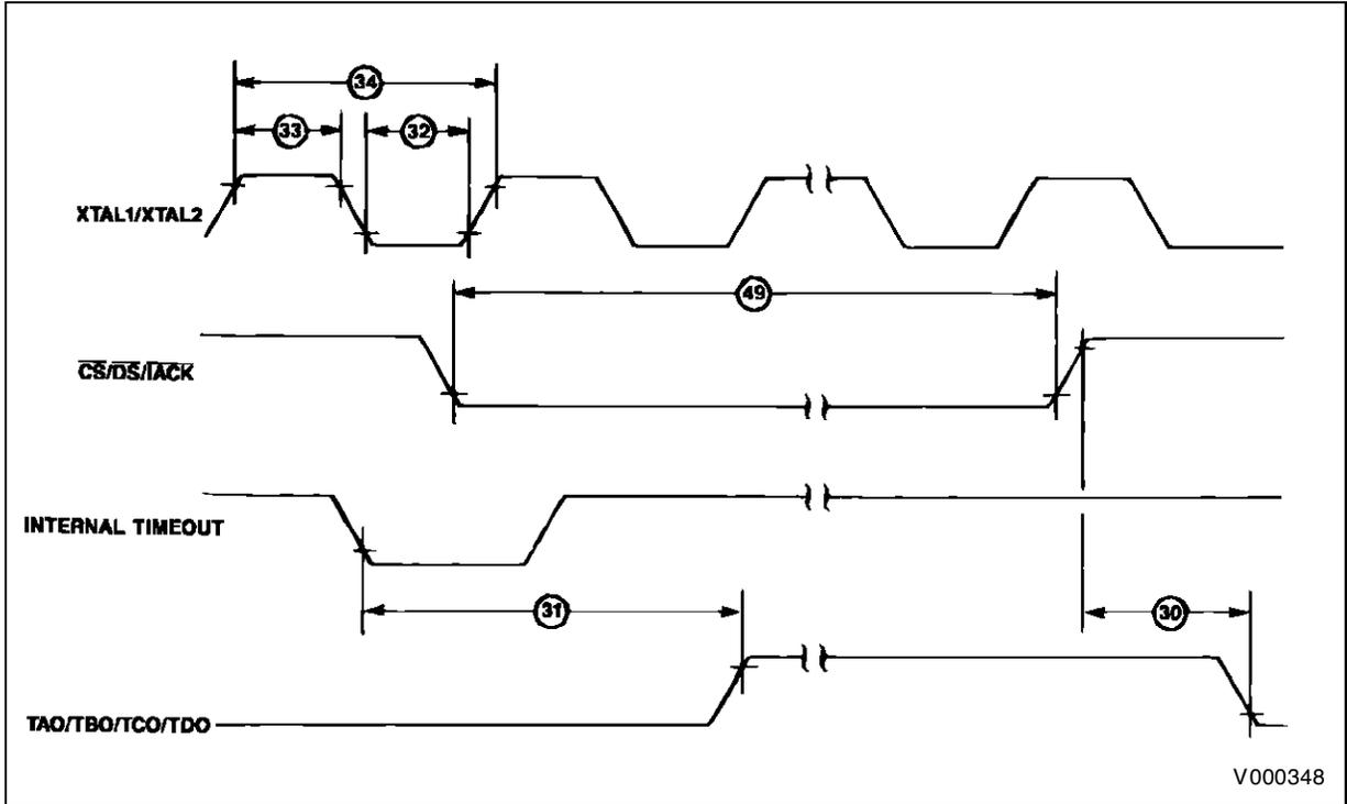
Figure 30 : Reset Timing.
