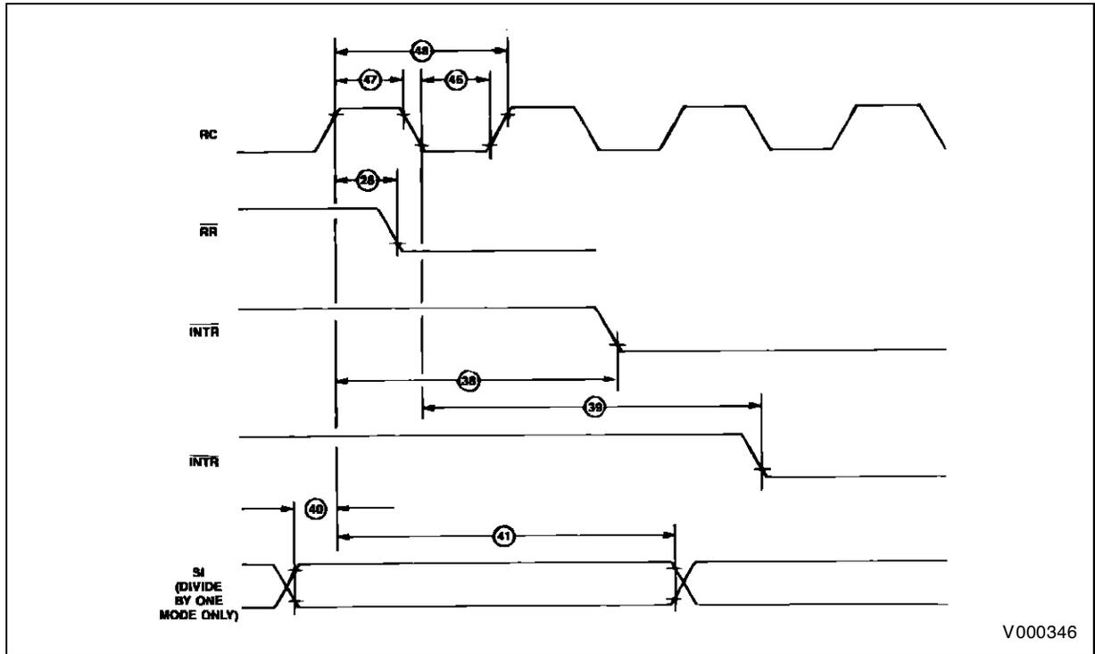
Figure 28 : Transmitter Timing.
