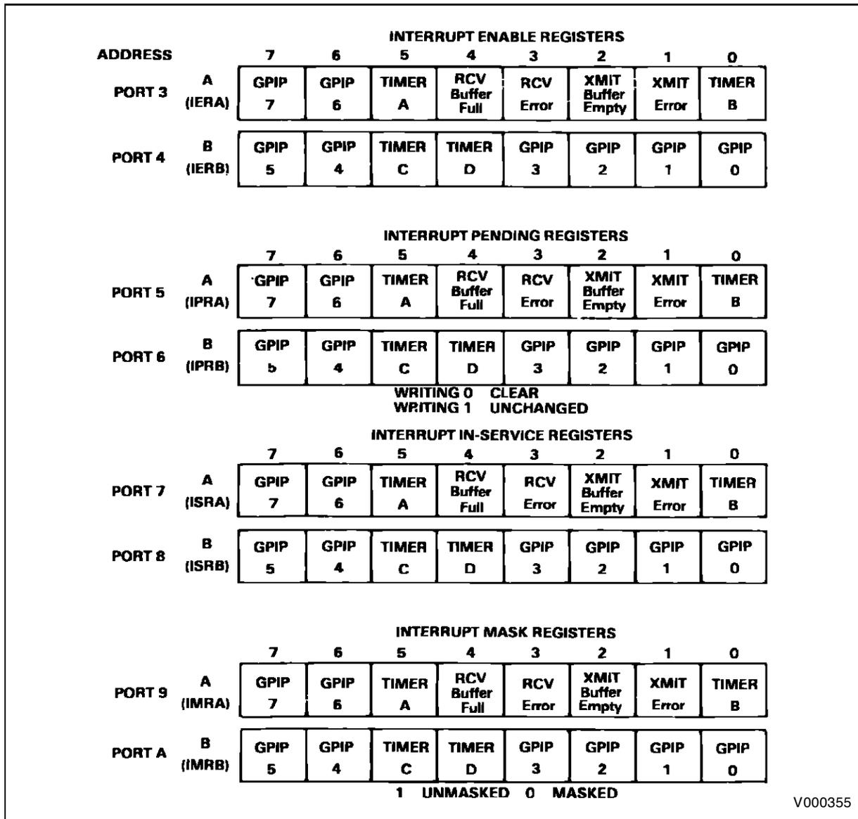
Figure 9 : Interrupt Control Register Definitions
