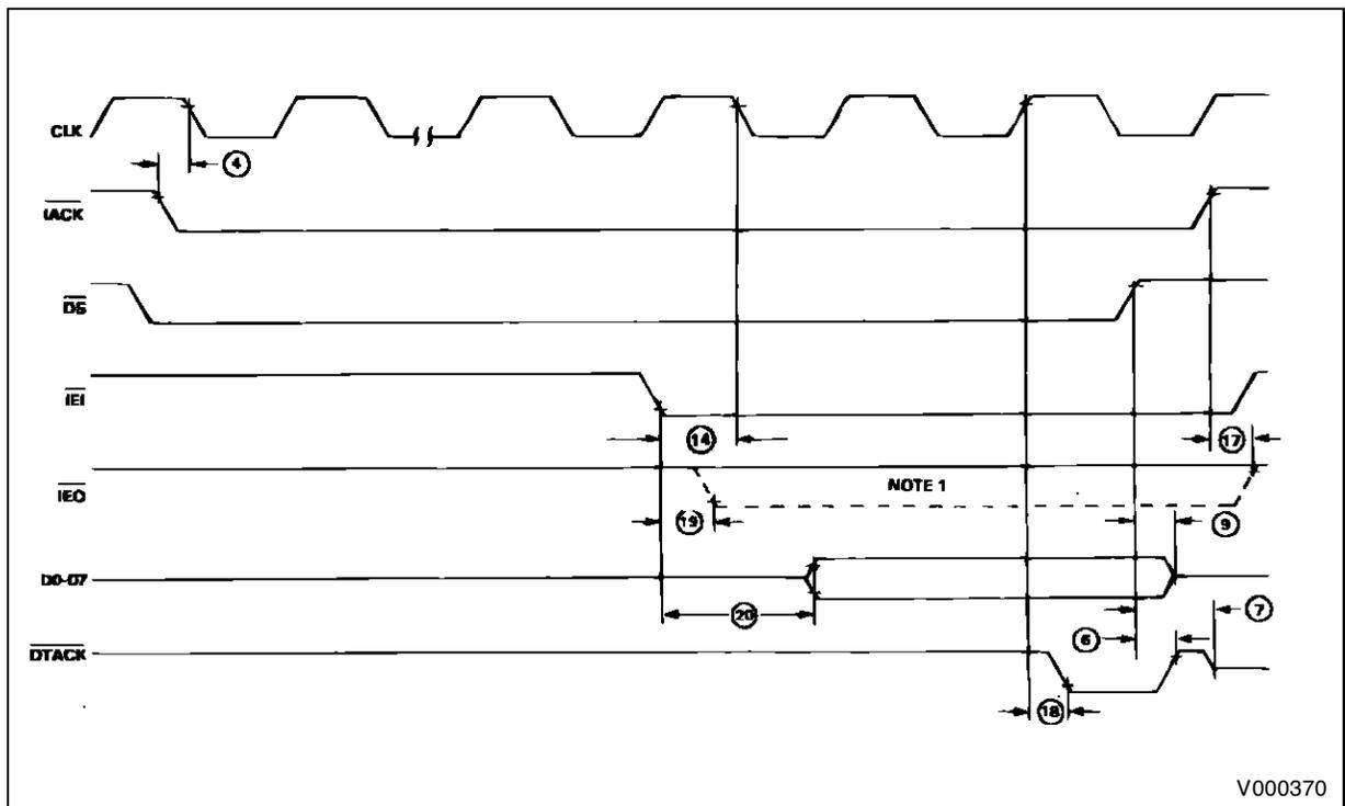
Note :  $\overline{CS}$  and  $\overline{IACK}$  must be a function of  $\overline{DS}$ .
