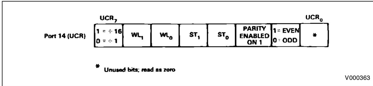
$\div 16/\div 1$  : When this bit is zero, data will be clocked into and out of the receiver and transmitter at the frequency of their respective clocks. When this bit is loaded with a one, data will be clocked into and out of the receiver and transmitter at one sixteenth the frequency of their respective clocks. Additionally, when placed in the divide by sixteen mode, the receiver data transition resynchronization logic will be enabled.
