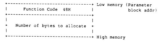
Long contains the number of bytes to allocate, or -1L (FFFFFFFF), which returns maximum available memory.
