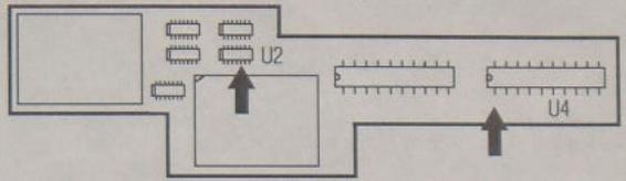
Remove the three pin connector, the red clip and the green clip from the CyReL Cal Tamaran wires (if still present). Connect the wire <E> (Rev.A Cal Tamaran boards) or wire <A> (Rev.B Cal Tamaran boards) to pin 18 of U4 as shown here:
