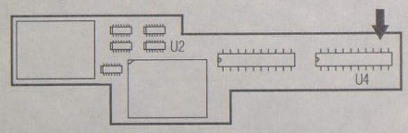
Take a 74F00 (or 74F04, but notice the different pin layout on the F04!). Solder it in piggyback fashion ontop of U4, connecting pin 14 (VCC) of the 74F00 to pin 20 of U4 and pin 7 (GND) of the 74F00 to pin 10 of U4. Keep these wires short. Connect pin 8 of the 74F00 to
