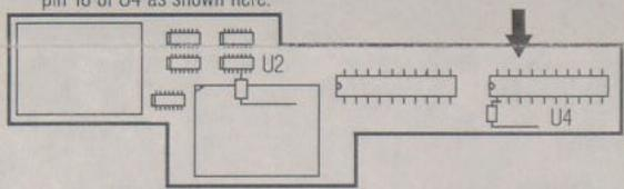
Remove wire 4B (Rev.A Callamaran boards) or wire 4D Rev.B Callamaran boards) from the Callamaran and solder the third 33 ohms resistor to the same connection as the wire before. Then, solder the wire back to the other end of this 33 ohms resistor. Take the free end of this wire and solder it to the 33 ohms resistor on pin 1 of U4.
