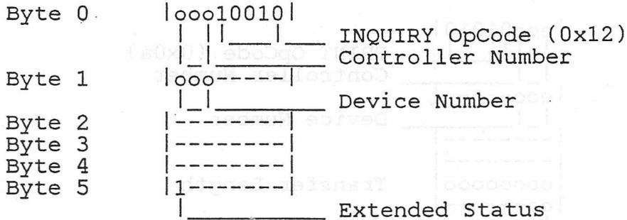
If byte 5 bit 7 is not set, then an Invalid Operation Code error is returned. Since the controller can not DMA data back to the host, the following Identification List is returned using the EXTENDED STATUS PHASE. Please note that a null Status Byte is returned before this operation.
