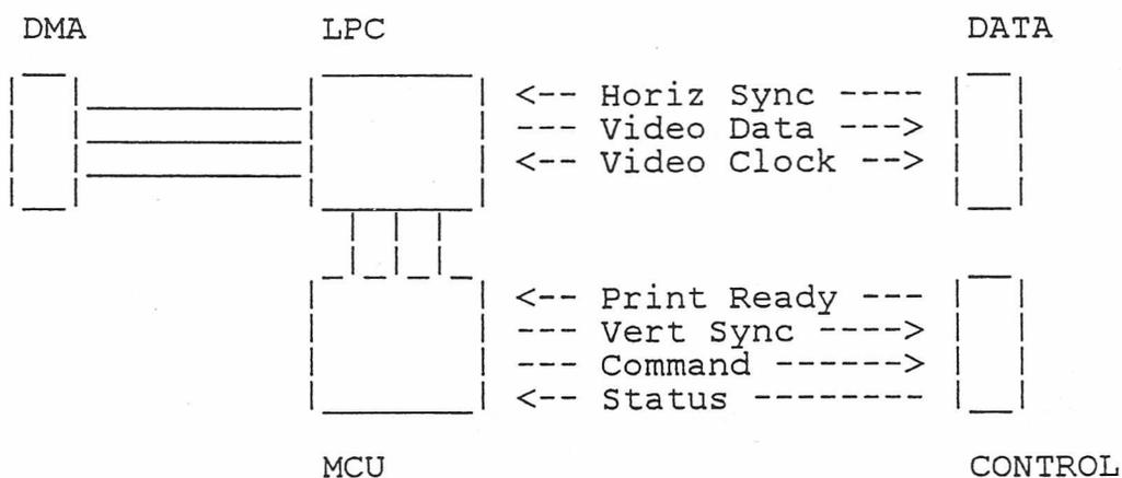
Bus communication follows a defined host-initiated dialog sequence consisting of a COMMAND PHASE, DATA OUT PHASE, and STATUS PHASE. Data transfers are asynchronous and follow a Data Request / Acknowledge handshake protocol, with one byte of data transferred during each handshake.
