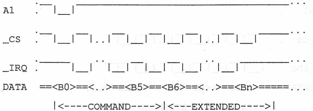
Please note that after writing each command byte, the host must wait a minimum of 20 microseconds before testing the state of IRQ (see Appendix). The controller does not raise IRQ on the falling edge of CS.
