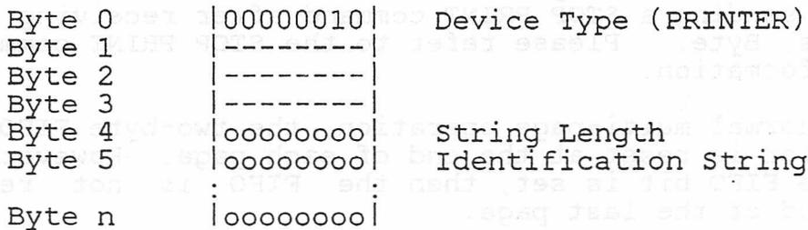
The Identification String contains ASCII characters describing the printer class, controller revision number, and controller manufacturer. The string is separated by colons and terminated by a space (for example "PAGE PRINTER:SLMC804v1.1:ATARI ").
