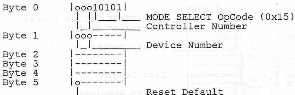
Please refer to the MODE SENSE command for a detailed description of the Parameter List. The host should perform a MODE SENSE before MODE SELECT in order to obtain the current controller state (except for Reset Default, where the current state is obliterated).
