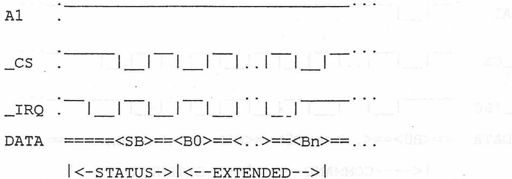
Please note that after reading each status byte, the host must wait a minimum of 20 microseconds before testing the state of IRQ (see Appendix). The controller does not raise IRQ on the falling edge of CS.
