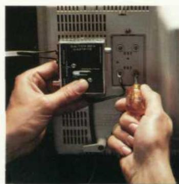
Locate the twin-lead cable marked *TV* on the TV Switch Box. Connect it to the two VHF terminals on your TV. Peel off the protective cover from the self-adhesive yellow square on the back of the Switch Box and attach to the back of your TV. If your TV was connected to a flat, twin-lead (300 Ohm) cable, you have finished installing the TV Switch Box.
