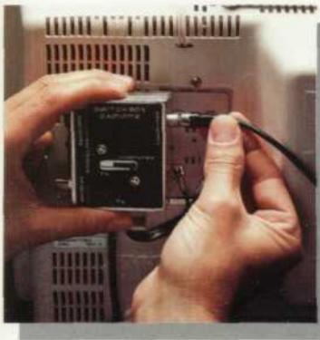
Plug the cord from the back of the computer into the socket on the Switch Box labeled *Computer* or *Game*. Set the TV Switch Box to the Computer position. Turn on your TV and tune to Channel 2 or 3, whichever is weaker in your area.
