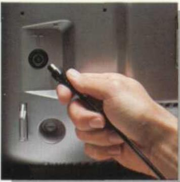
Plug the round cord that comes from the back of the computer console into the antenna socket of your television. Turn on your television and tune it to channel 36 (PAL/UK) or channel 4 (PAL).
