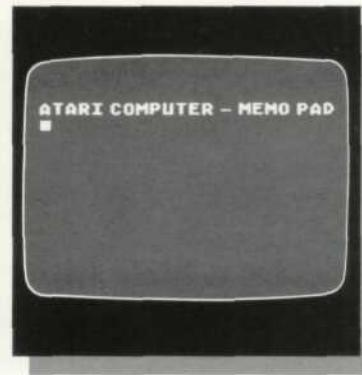
With the cartridge door closed, push the Power Switch on the side panel to the "ON" position. The words ATARI COMPUTER-MEMO PAD should appear on the screen.
