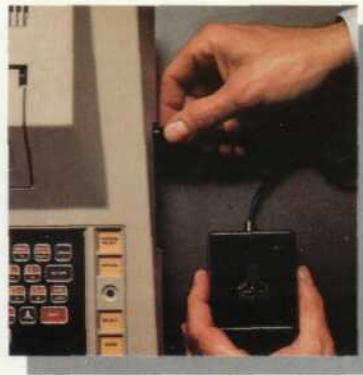
Set the Channel Select switch on back of computer to the same channel.
