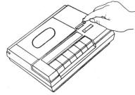
Type CSAVE and press RETURN on the computer. You'll hear two beeps to remind you to press RECORD on the program recorder. Finally, press RETURN again on the computer. The cassette will begin recording.
