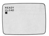
After pressing the PLAY button on the program recorder, press the RETURN key again on the computer console. The cassette tape will start turning and your computer will load the program into its memory.
