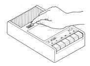
Type CSAVE and press RETURN on the computer. You'll hear two beeps to remind you to press RECORD on the program recorder. Finally, press RETURN again on the computer. The cassette will begin recording.
