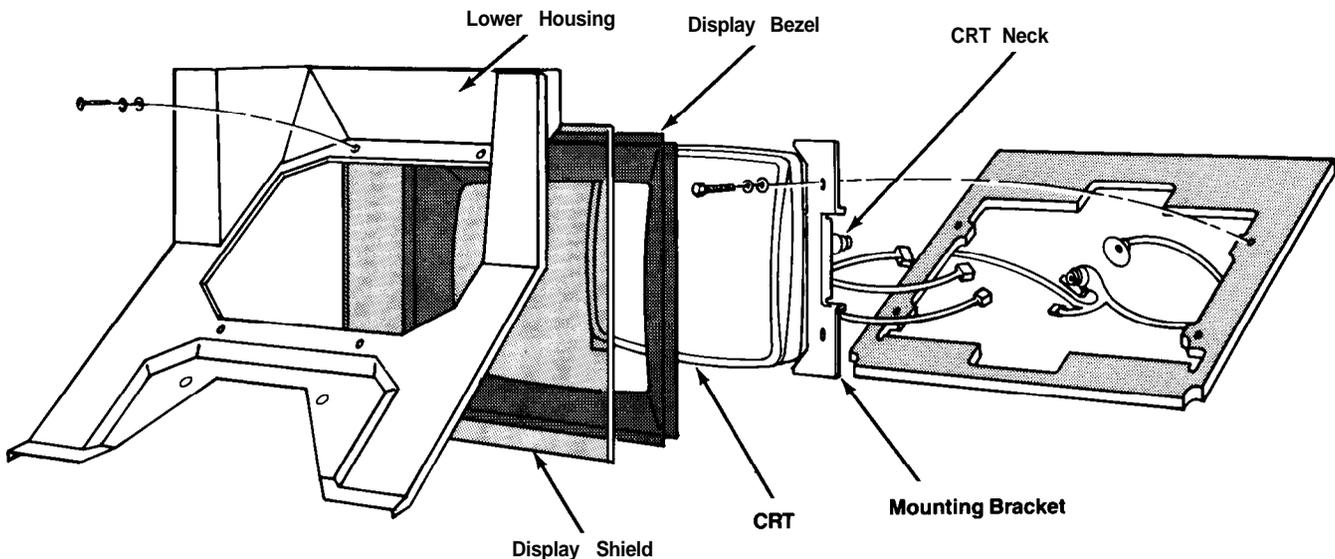
Figure 4-3 Removing the CRT Assembly
