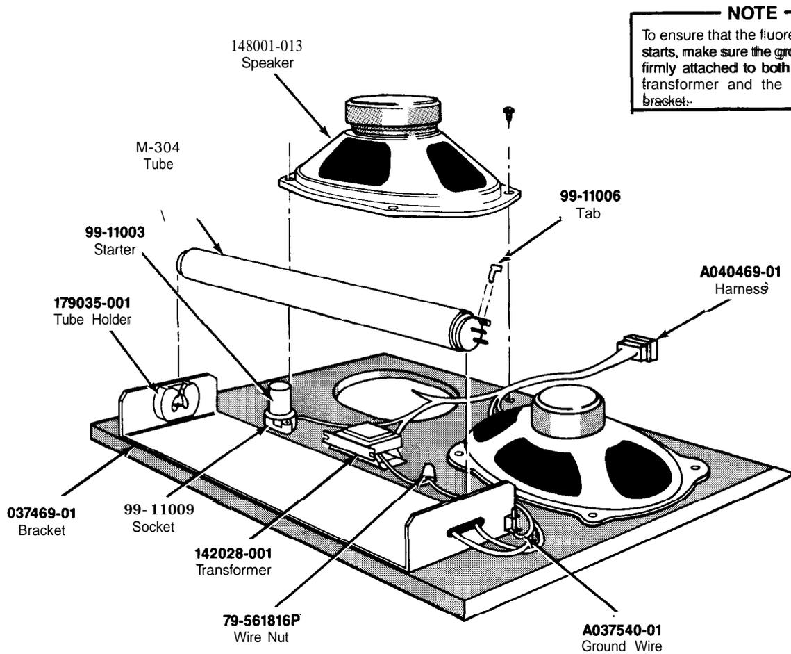
**Figure 5-4 Fluorescent Tube and Speaker Assembly
