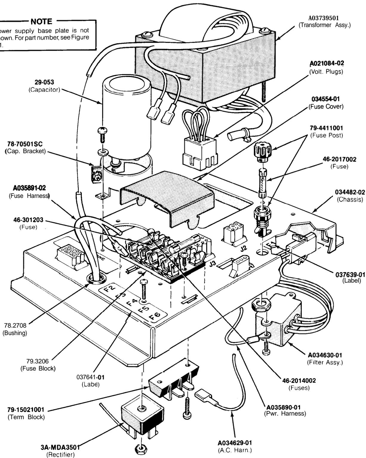
**Figure 5-8 Power Supply Assembly
