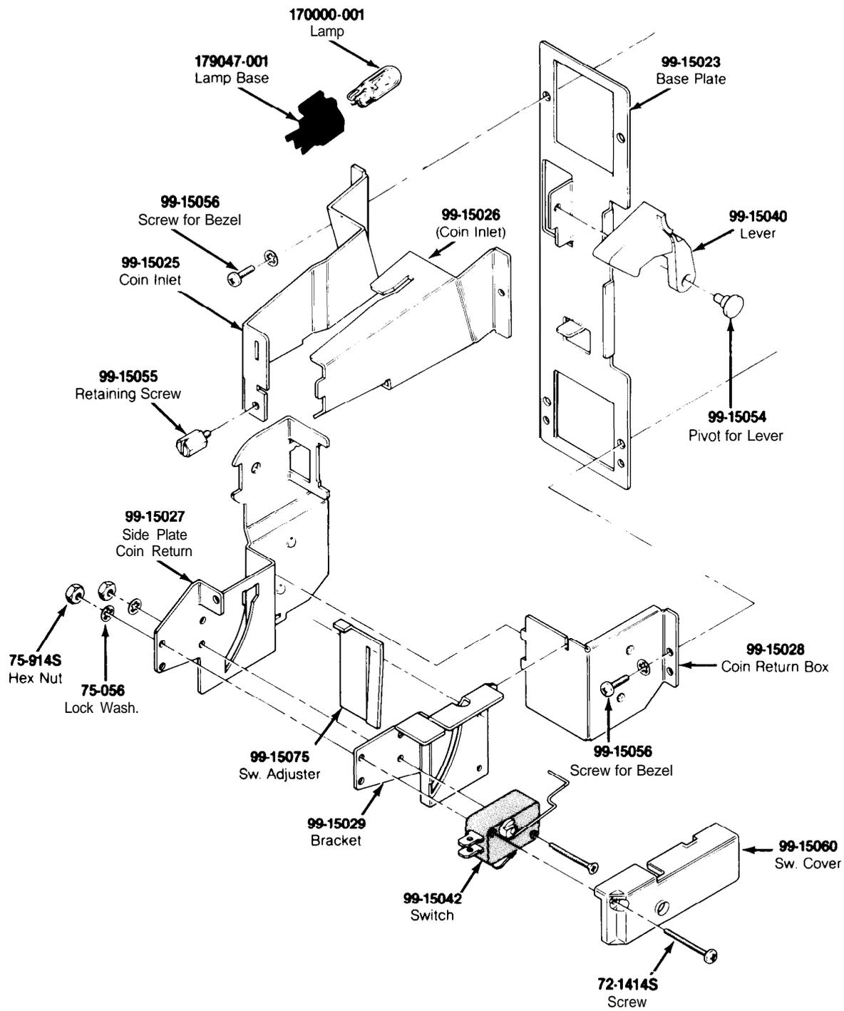
Figure 5-6 Vertically Mounted Coin Door
