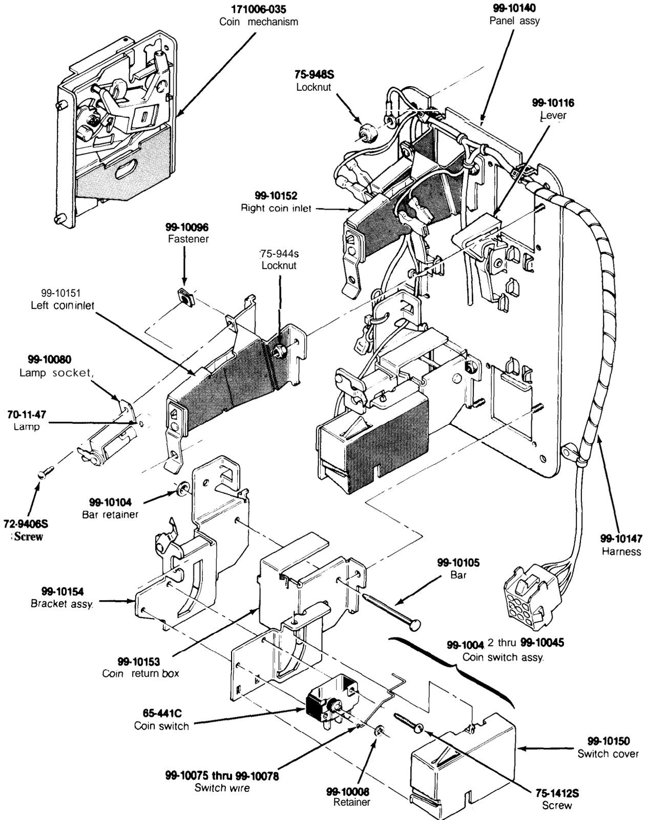
Figure 5-7 American-Made Coin-Door Assembly
