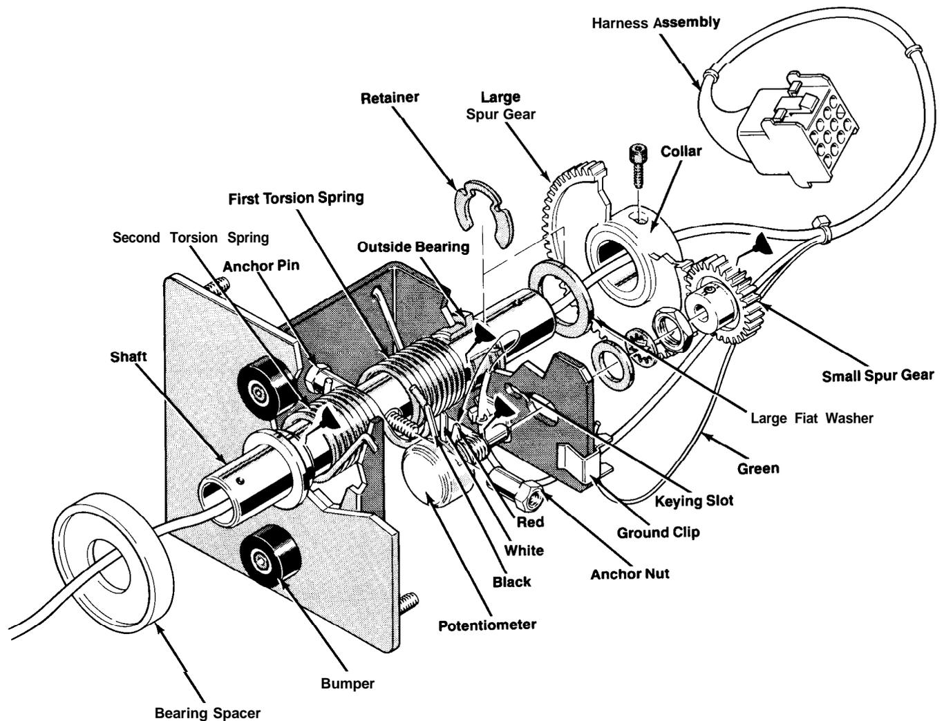
**Figure 4-2 Steering Assembly**
