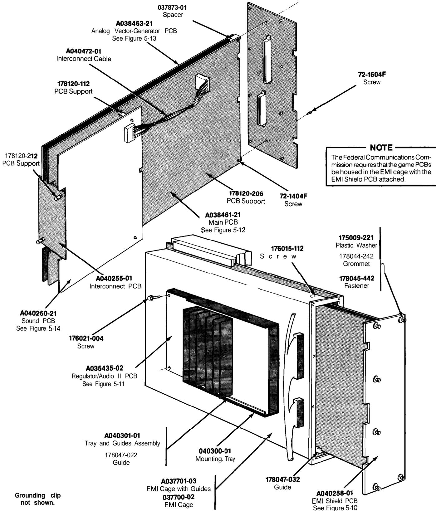
**Figure 5-9A PCB Mounting Hardware
