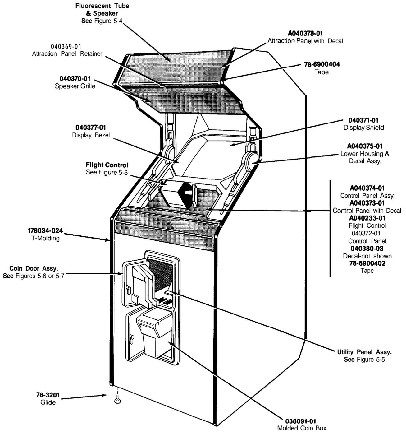
**Figure 5-1A Cabinet-Mounted Assemblies**
