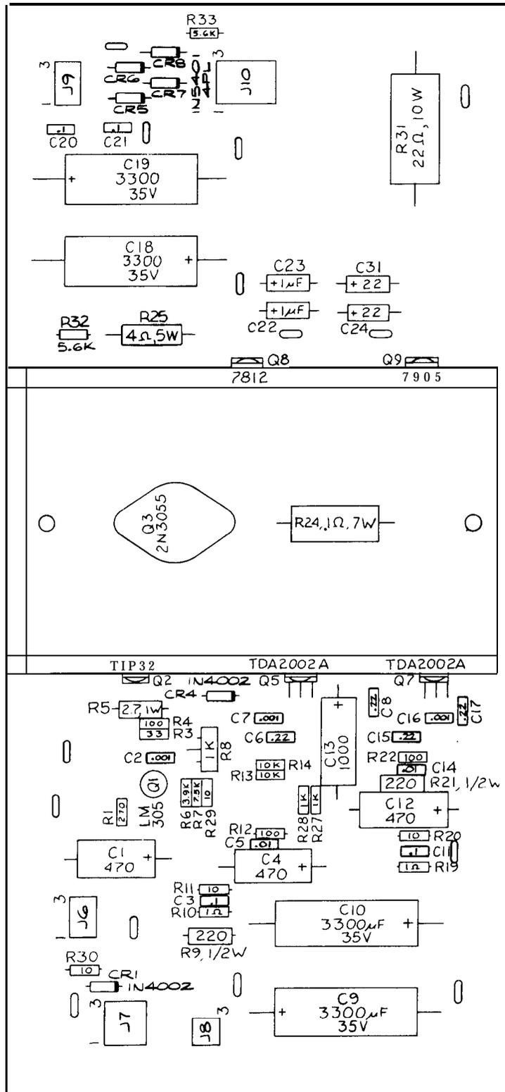
**Figure 5-11 Regulator/Audio II PCB Assembly**
