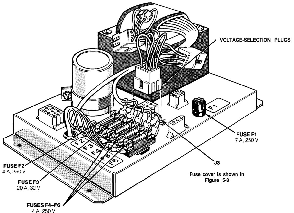
Figure 1-2 Voltage-Selection Plug and Fuse Locations
