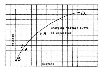
Therefore, when a line appears on the CRT, it is actually only part (section A-B, Figure C) of the entire path taken between the beginning and ending points of the vector (C-D). The section of A-B is chosen as the most linear portion of the charge curve, and illuminated
