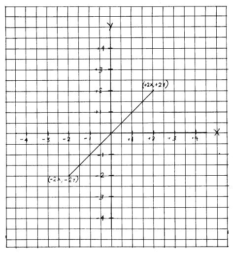
A line is drawn by programming a beginning and ending point of the line to be drawn, and forcing the cathode beam to travel between these two points, illuminating the entire path of phosphorus on the CRT. The angle of the line, the position of the line, and the length of the line are determined simultaneously, and simply, by selecting the proper voltage levels for the beginning and ending points of the line.
