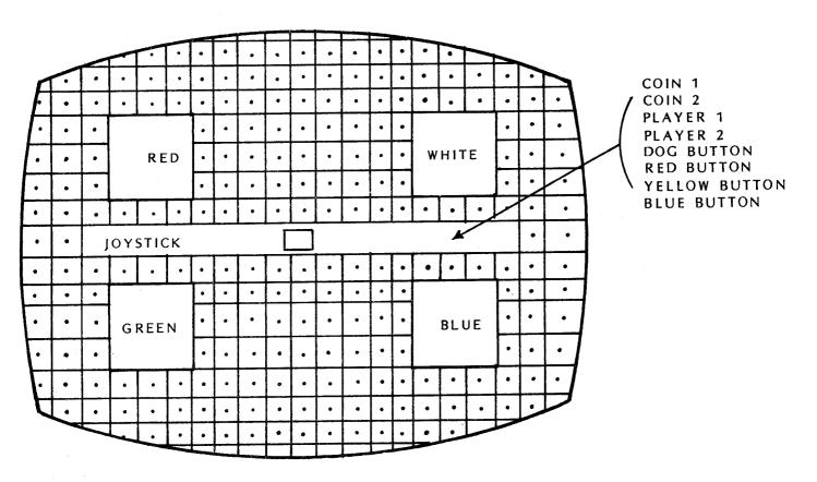
The grid pattern tests your screen for any distortion or convergence.
