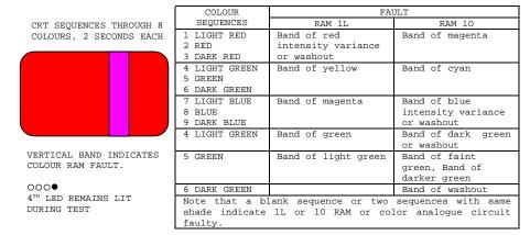
Tests 5 and 7 provide sequential subtests. To stop automatic cycling set switch to MANUAL/DOWN. Depress ADVANCE in MANUAL-DOWN to step through subtests.
