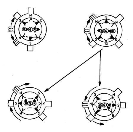
Figure 5-2, 6-Pole Convergence Magnets
