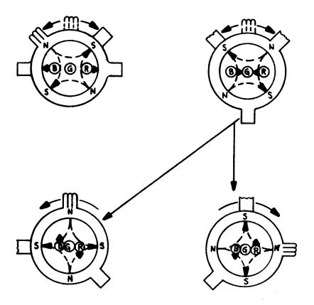
Figure 5-1, 4-Pole Convergence Magnets
