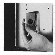
Disconnect the television antenna from the antenna socket on the back of you television set
