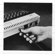
Connect one end of the RF Cable to the socket marked "television" on the back of the computer.
