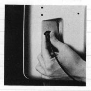
Connect the other end of the RF Cable to the antenna socket on the back of your television set.
