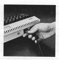
Connect one end of the monitor cable 5-pin plug (not included with Purchase) to the socket marked "monitor" on the back of the computer.
