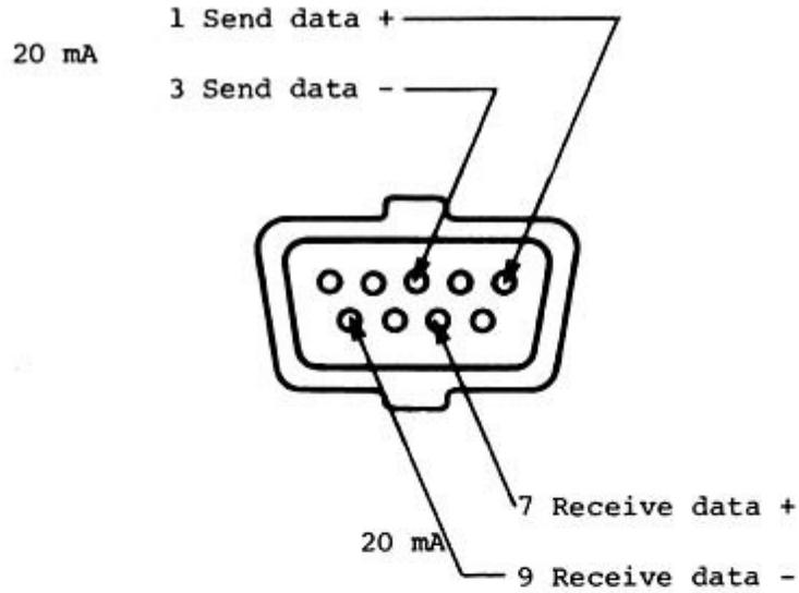
Figure 4. Hook-up of Serial Port No. 4 used with a 20 mA loop device.
