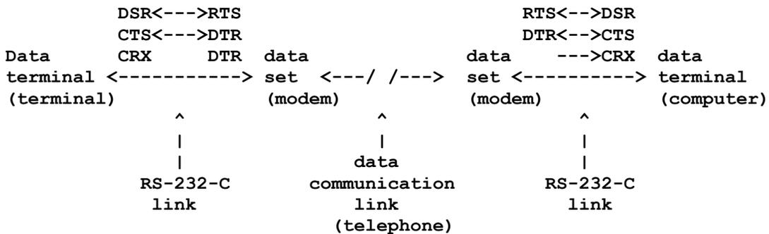
The data-set/data-terminal distinction should be kept in mind because the RS-232-C interface is DIRECTIONAL. That is, each line in an RS-232-C interface has a direction--one device drives the line (sends information) and the other receives the information. Each line in an RS-232-C interface is defined as being driven by either the data-set end or the data-terminal end.
