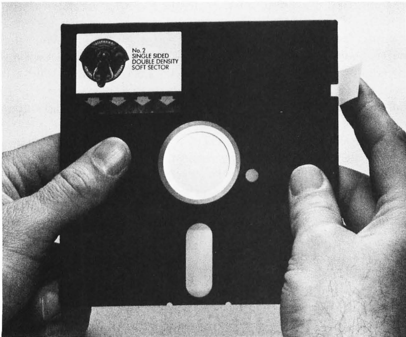
Figure 10.4: By covering the write-protect notch, you can keep the disk drive from erasing information.
